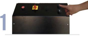
Press the UP button to raise both platforms at maximum height
