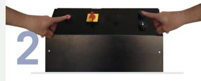
Simultaneously press the UP button and the off-photocell button for 3 minutes to complete the purge of the hydraulic circuit
